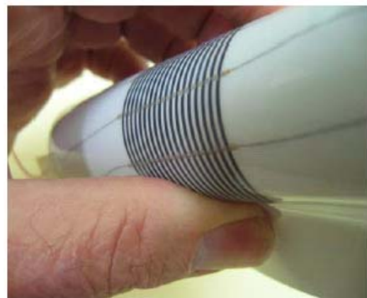
Figure 1: Flexible 12 volt elongate module
