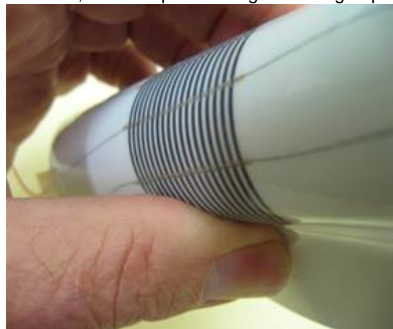
Figure 12. A flexible SLIVER module constructed from flexible Raft sub-
