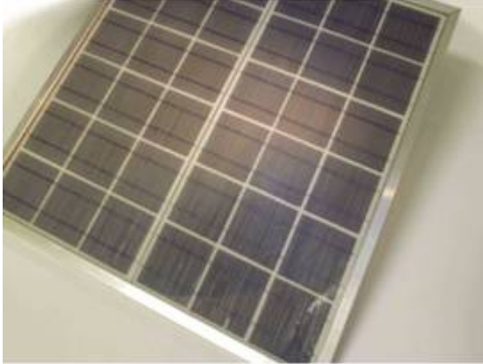
Figure 11. A SLIVER module constructed using Raft sub-modules.
