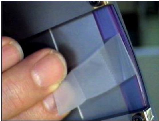
Figure 4. Transfer of SLIVER cells to a single-stack cassette.
