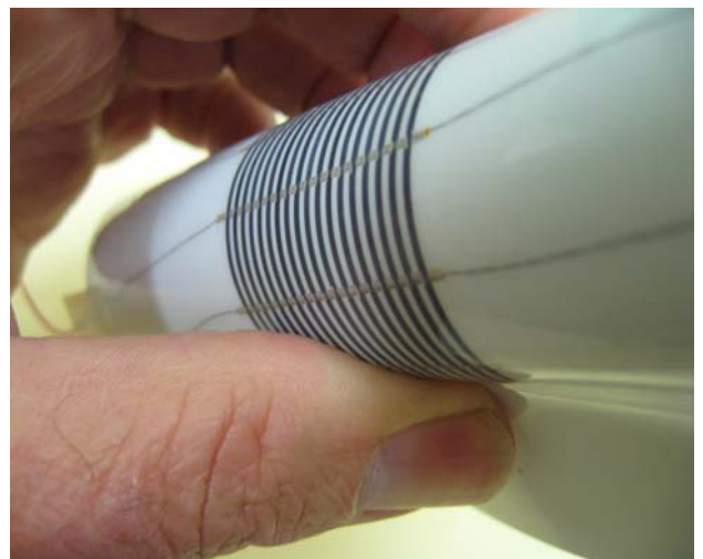
Figure 8. A flexible Sliver® module constructed from flexible Raft sub-modules.
