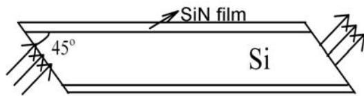
Figure 1: MIR measurement. Light enters the edges of the sample, which have been cut at 45°, and is trapped, interacting with the surfaces ~20 times before escaping.
